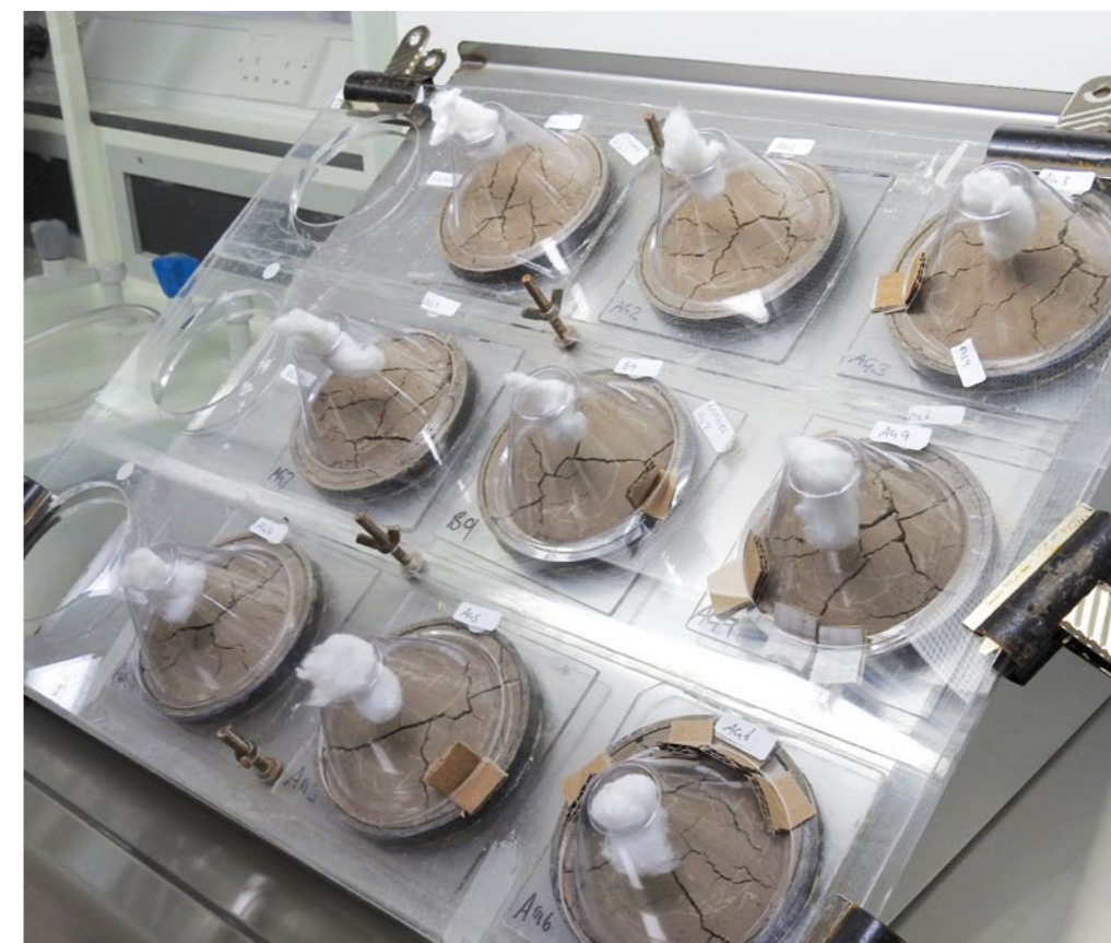
◀ Testing the durability of insecticides on alternative mud surfaces.
